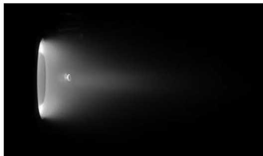
Fig. 11 Hall-effect thruster operating with a well-structured plume at 3 A of anode current and 260 V using zinc propellant with an argon cathode.
