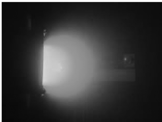
Fig. 6 Preliminary experiment showing a Hall-effect thruster operating using magnesium propellant and an argon cathode, with no attempt made to control the anode temperature and, hence, the mass flow rate.
